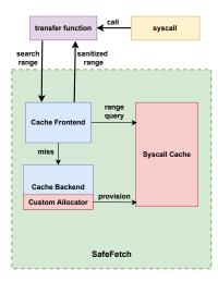
Figure 3: SafeFetch's high-level architecture.
