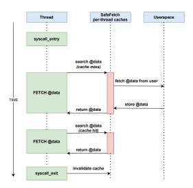
Figure 2: SafeFetch hindering a double-fetch exploit.
