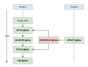
Figure 1: Workflow of a double-fetch exploit.
