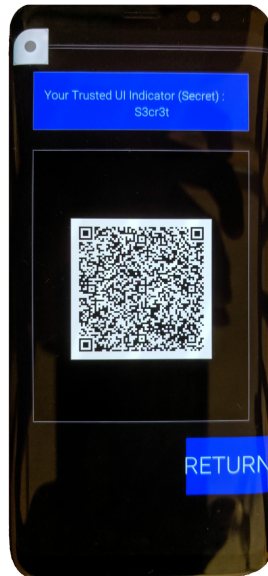
Figure 3.5. Registering with the bank by showing the QR code of public key on the trusted screen
