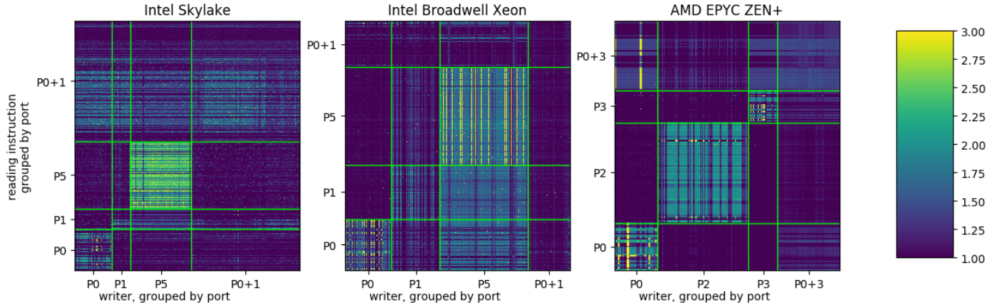
Fig. 2: Exhaustive map of instruction interference grouped by 4 different execution port sets on 3 different microarchitectures. For each microarchitecture, we visualize the matrix CC_{B,A} as constructed using Algorithm 1.
